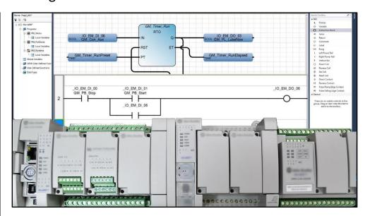
Nano Basics is designed for those students who have basic PLC knowledge and would like to learn how to setup, program, and troubleshoot the Allen-Bradley Micro800 line of Nano Programmable Controllers using Connected Components Workbench.
